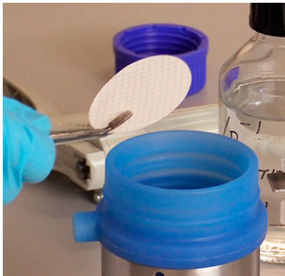
Figure 13. Placing the filter into the unit
