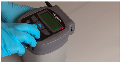
Figure 21. Operating the incubation unit
