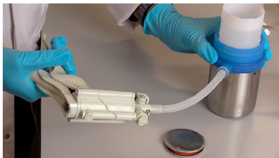
Figure 17. Operating the vacuum pump
